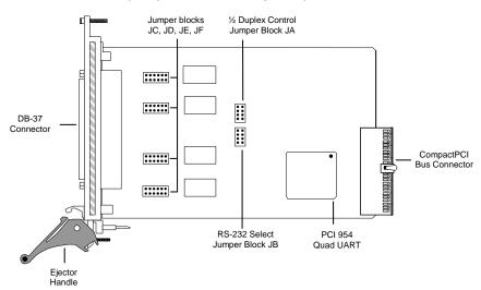
Figure 2: Titan/cPCI Model TN004 for compatibility with 64 bit systems
